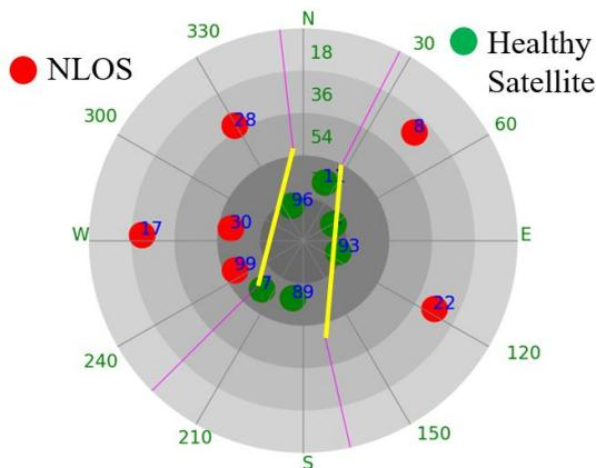
Fig.7 Skyplot indicating the satellites distribution during the dynamic experiment. Green circle represents the satellites that are healthy. Red circle denotes the NLOS satellites. Yellow line indicates the building surface boundary.
