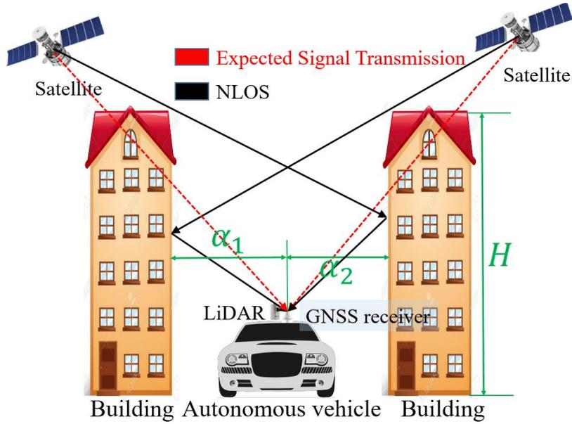
Fig.1 Illustration of NLOS receptions caused by surrounding buildings.
