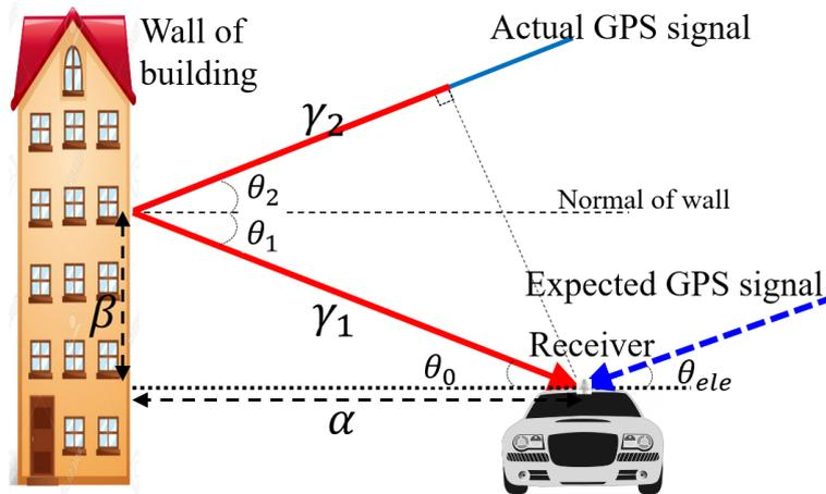
Fig.5 NLOS correction model. The signal is reflected by the building and received by receiver subsequently [9]
