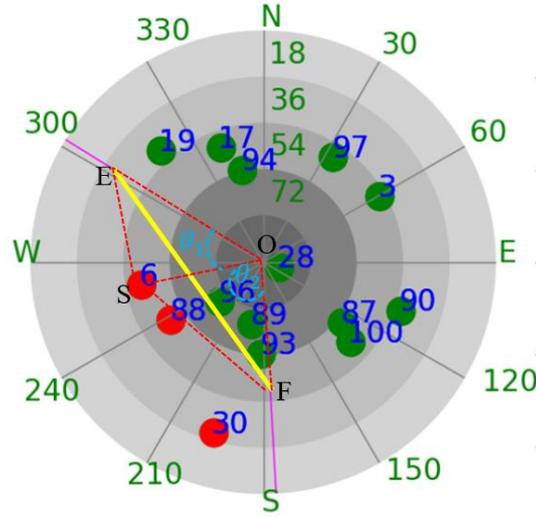
**Fig.4 Skyplot of GNSS satellites and detected building surface boundary. Green and red circles and the nearby numbers indicates satellites and corresponding PRNs. Line segment  $\overline{EF}$  indicates the boundary.**
