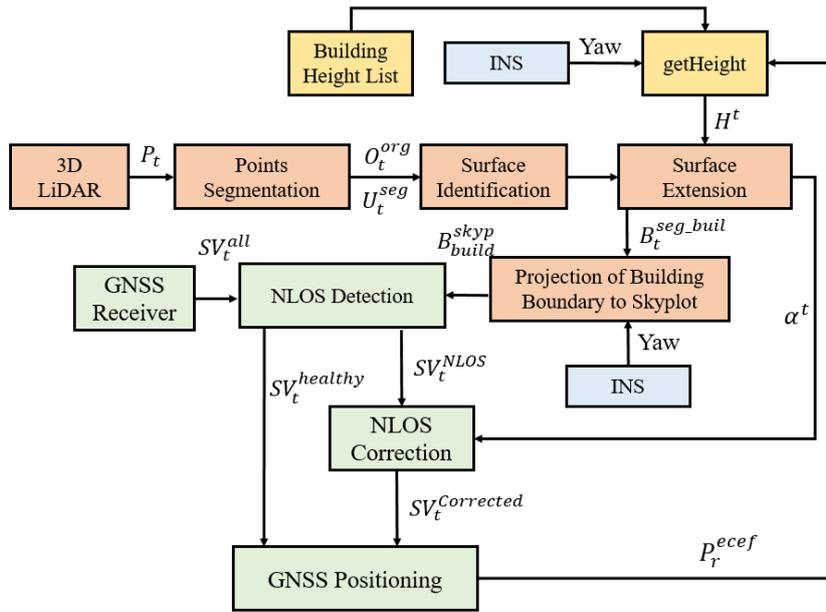
Fig.2 Illustration Overview of the proposed algorithm of NLOS correction and corresponding positioning flowchart. The main inputs are GNSS raw measurements and real time point clouds from 3D LiDAR. The auxiliary inputs are yaw angle from INS and building height from Google Maps.
