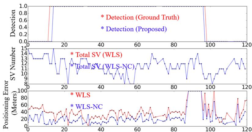
**Fig.8 Experimental results of WLS-ESF and WLS-ESF-NE, which depicted in red and blue dots, respectively. Top panel indicates the building surface detection result. Middle panel indicates the numbers of satellites used. Bottom panel indicates the 3D positioning errors.**
