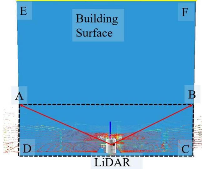
**Fig.3** Illustration of point sets segmentation and building surface identification. Blue box ABCD represents the initially detected building surface. Blue box CDEF represents the extended building surface.
