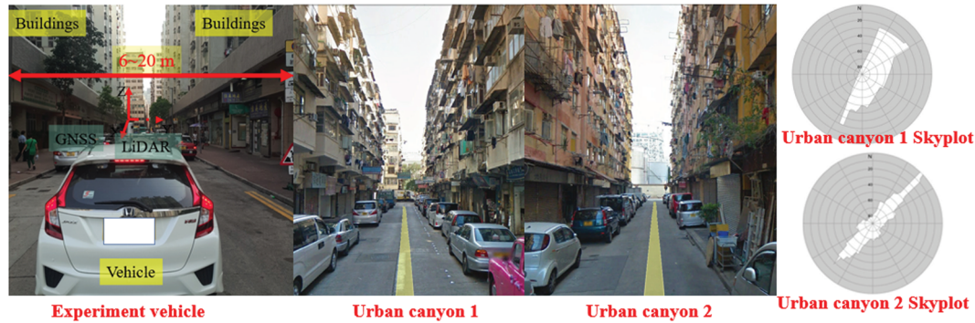
FIGURE 7 The sensors setup of the vehicle and tested environment: GNSS and LiDAR sensors are installed on the top of the vehicle shown in the left side of the figure. The two tested urban scenarios are shown in the middle of the figures. The Skyplot of the two experiments is shown in the right side of the figure [Color figure can be viewed at wileyonlinelibrary.com and www.ion.org ]
