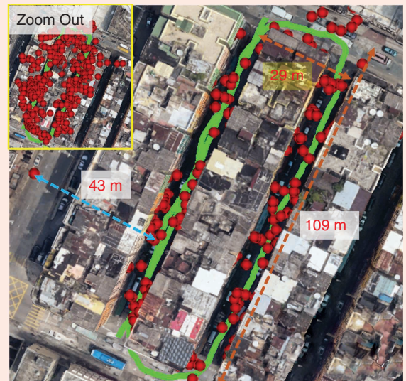
FIG 14 Experiment 2: the trajectory of the vehicle is indicated by the green curve, while the red circles denote the object-detection-aided GNSS-positioning results. The background image is captured from Google Earth.
