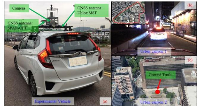
**Fig. 4** The sensor setup of the experimental vehicle and evaluated scenarios. (a) sensor setup of the experimental vehicle. (b) the experimental scene with tall buildings in urban canyon 1. (c) the experimental scene in urban canyon 2.
