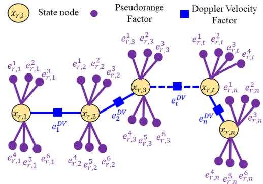
Fig. 2 The purple circle denotes the pseudorange factor (e.g  $e_{r,t}^s$ ). The blue shaded rectangle represents the Doppler velocity factor (e.g  $e_t^{DV}$ ). The yellow shaded circle stands for the state of the GNSS receiver.
